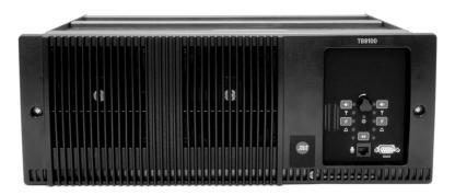
The TB8100 is a software-controlled base station system (BSS) which is designed for operation on most standard frequency ranges<sup>1</sup>. It makes extensive use of digital and DSP technology. Many operating parameters such as channel spacing, audio bandwidth, signalling, etc. are controlled by software. It is also capable of generating alarms for remote monitoring.
